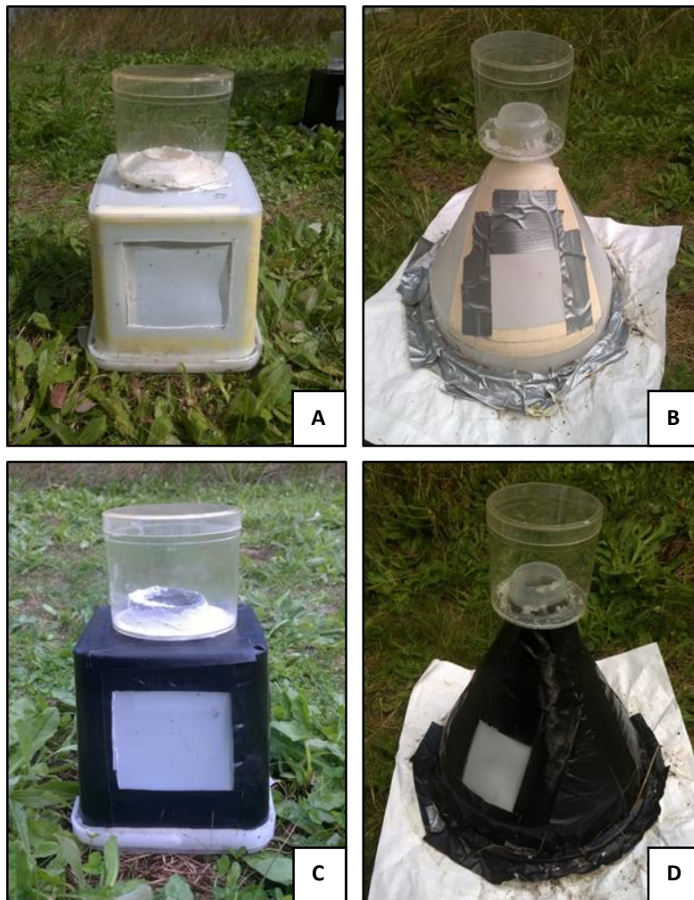
Fig. 2: The different traps used in this experiments. A, C: box-like electors, B, D: funnel-electors. The traps with the same shape shared the same structure. The different colors were applied by covering originally white electors with black plastic foil. The white lateral squares are mesh-covered aeration windows, the transparent plastic tin served as collection container. The letters A to D were used as a code designation.
